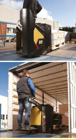
(Pictured from top ) The **NPF25N2** features a fixed platform to offer more protection for the driver.
